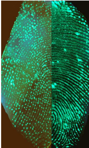
Figure 13: Illustration of fluorescence and ridge detail of a developed finger mark observed on a metal knife. Left side: image taken following water-based BY40 treatment. Right side: Image taken following ethanol BY40 treatment.
